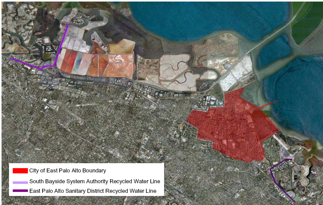
Figure 4-10 EPASD and SBSA Recycled Water Lines
