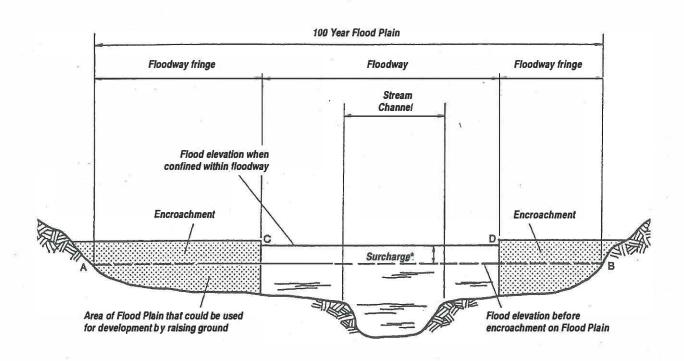
Line AB is the Flood Elevation before encroachment
