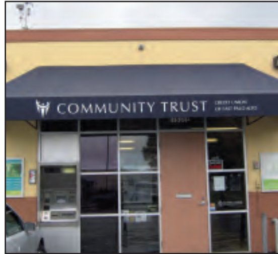
ENCOURAGED! Place the text of an awning sign on the valence portion of the awning
