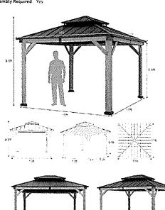
Four - Pre-Fabricated Gazebos - 10'X12' CEDAR (3 Sides, back and left and right sides to be enclosed)
