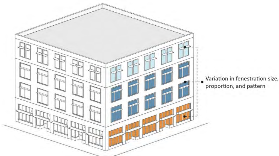
Figure 6-18: Examples of Base/Middle/Top Building Variation
