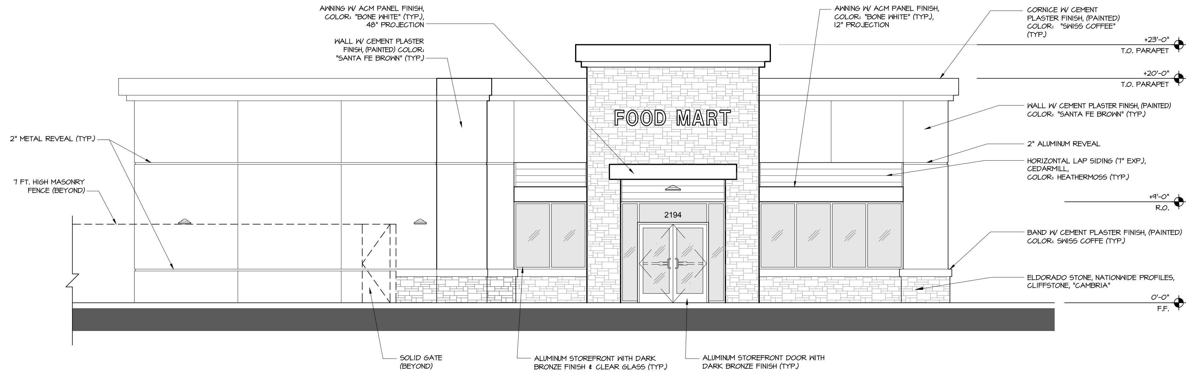
A NORTHWEST BUILDING ELEVATION (FACING UNIVERSITY AVE.) 3/16" = 1'-0"
