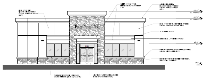
NORTHWEST BUILDING ELEVATION (FACING UNIVERSITY AVE.) Scale: 1/8" = 1'-0"
