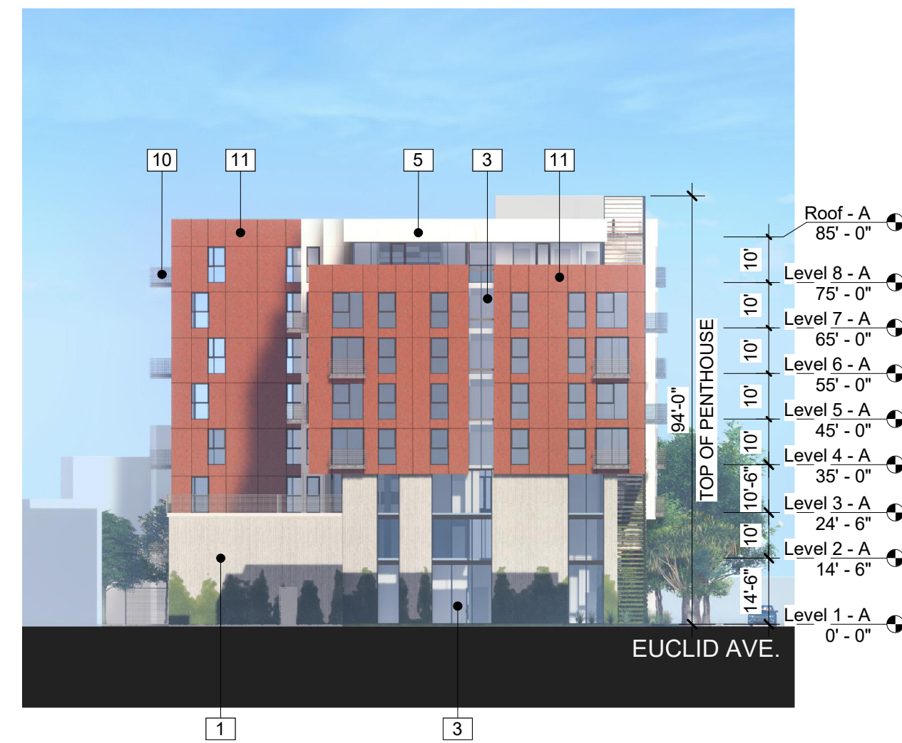
4 BUILDING A - SOUTH ELEVATION Copy 1 1" = 30'-0"
