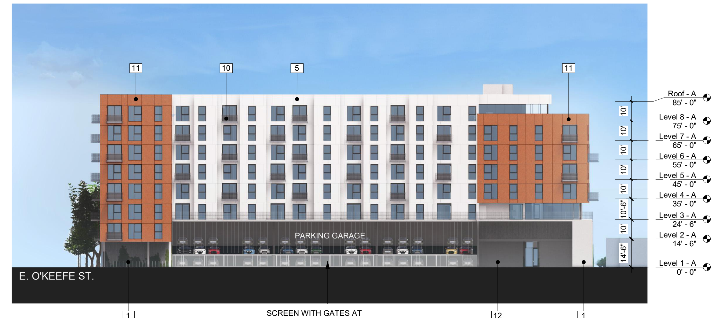
3 BUILDING A - WEST ELEVATION Copy 1 1" = 30'-0"
