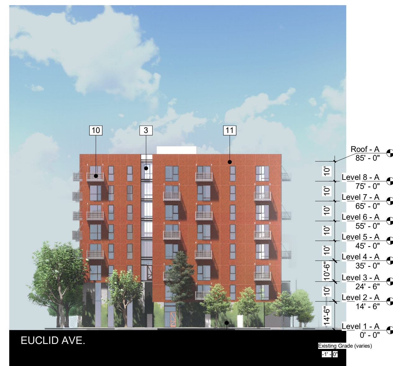
2 East O'Keefe St. Elevation - West Building 1" = 30'-0"
